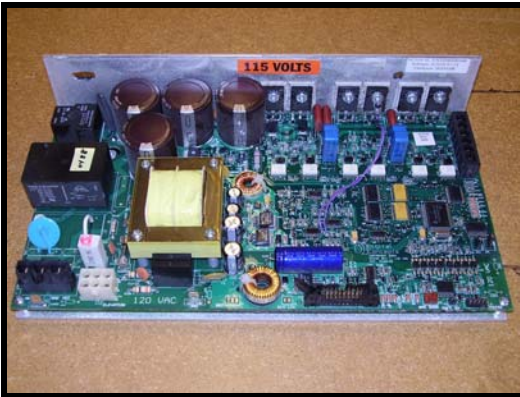
Part Number: SJFD06003A Description: Motor Controller ACD3X, 110v (T5x) Drawing Number: M08
