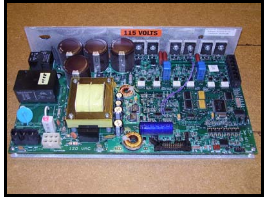
Part Number: SJFD06003A Description: Motor Controller ACD3X (T5x) Drawing Number: M08
